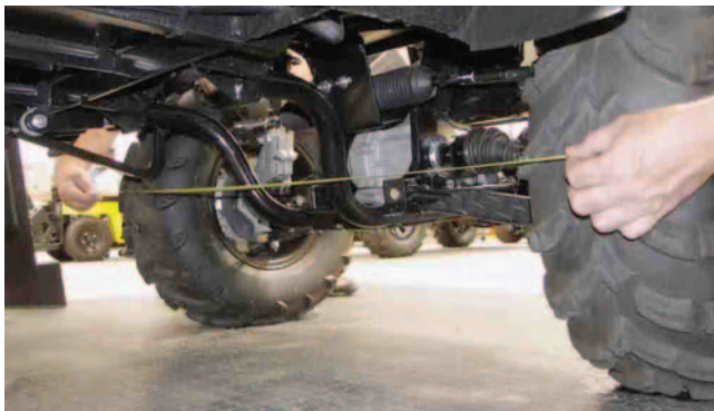
Fig. 15 Wheel Alignment Rear of Front Tires
