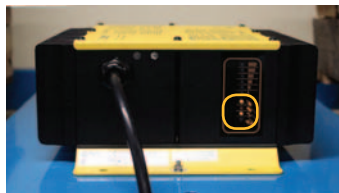
Figure 6: Bulk charge indicator displays charge profiles 7 and above.
