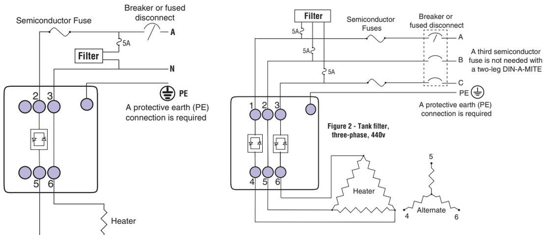
⚠ WARNING: Tank filters may suppress desirable communications carried on power lines in the 150 to 250 KHz region. The filters may suppress carrier current such as that used for infant monitors and medical alert systems. Verify that suppressed carrier current or other desirable communications on power lines creates no hazard to people or property. Failure to observe this warning could result in damage to property, and or injury to death for personnel.
