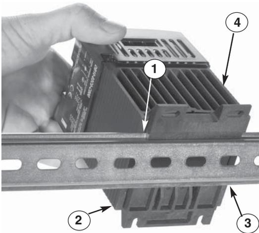
1. Push the unit in and down to catch the rail hook on top of the rail.
