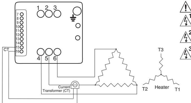
**3-phase, 3-leg Current Transformer Wiring**
