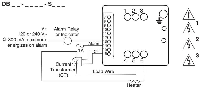
The Watlow DIN-A-MITE alarm option provides a common alarm output for shorted SCR conditions. **This is a non-latching alarm.**
