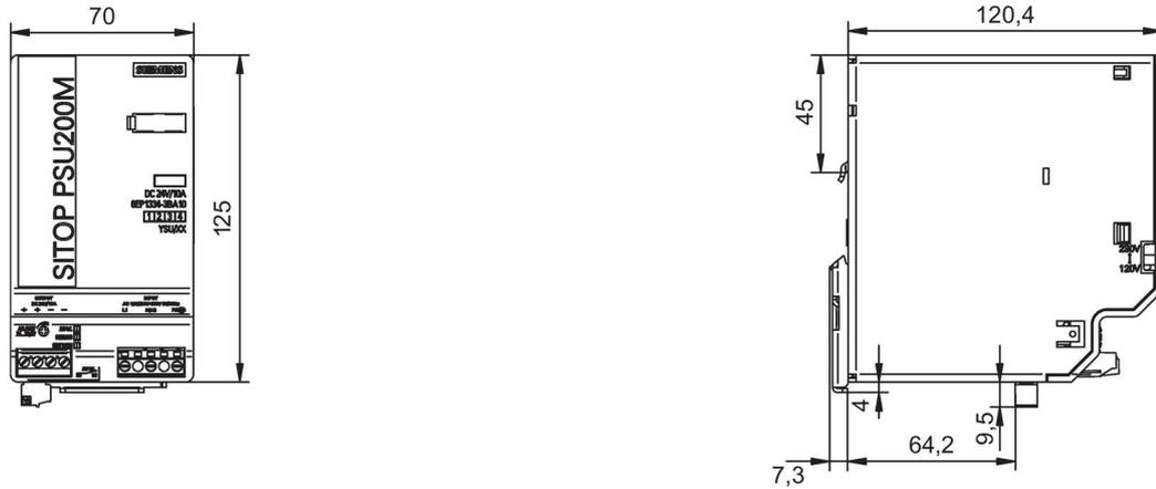
Figure 2-12 Dimension drawing, 6EP1333-3BA10 and 6EP1334-3BA10 (example, 6EP1334-3BA10)
