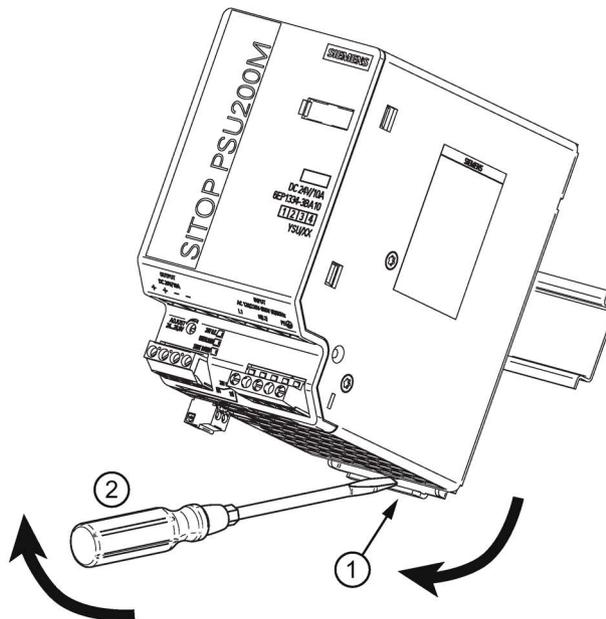
Figure 3-1 Removal (example, 6EP1334-3BA10)
