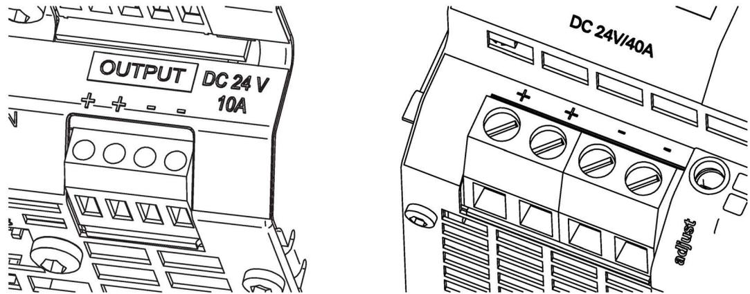
Figure 5-2 Output connection (example, 6EP1334-3BA10 and 6EP1337-3BA00)
