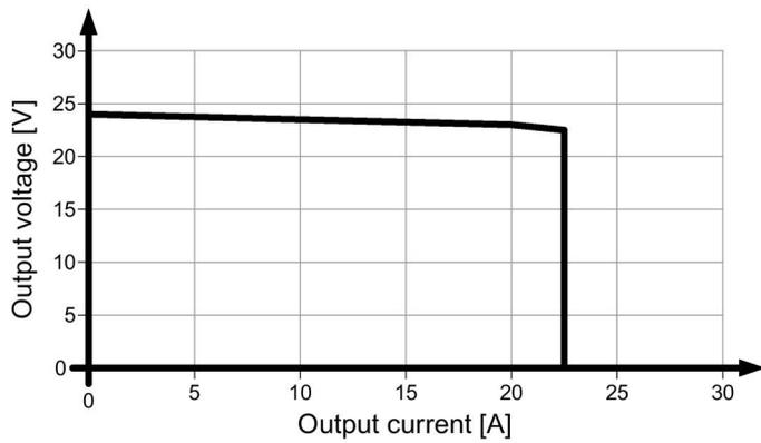
Figure 6-12 6EP1336-3BA00 parallel operation output characteristic
