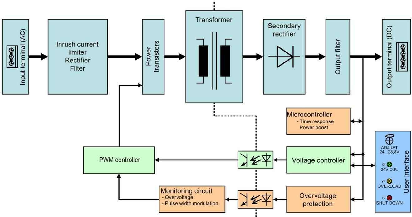
Figure 2-11 Block diagram for 6EP1336-3BA00 and 6EP1337-3BA00
