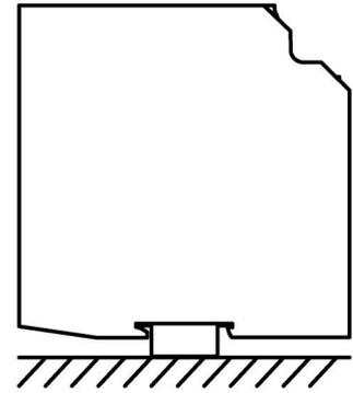
Figure 4-14 6EP1334-3BA10 mounting position (4)
