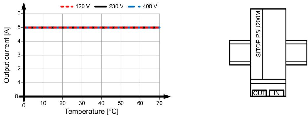
Figure 4-1 6EP1333-3BA10 output current for a standard mounting position
