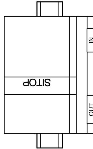
Figure 4-16 6EP1336-3BA00 mounting position (1)
