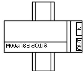
Figure 4-6 6EP1333-3BA10 mounting position (1)
