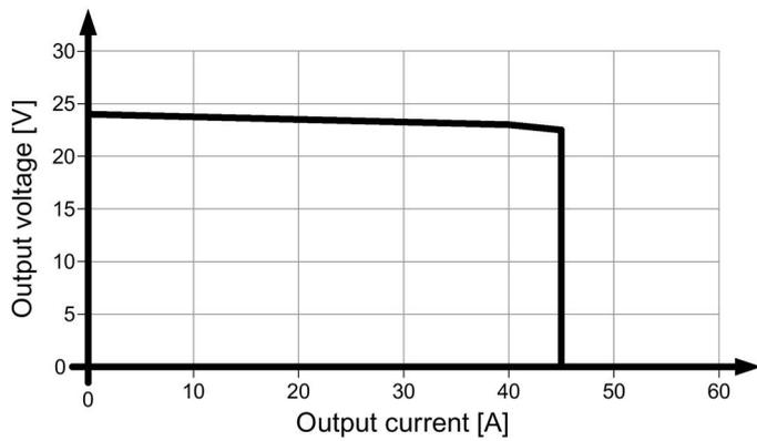
Figure 6-13 6EP1337-3BA00 parallel operation output characteristic
