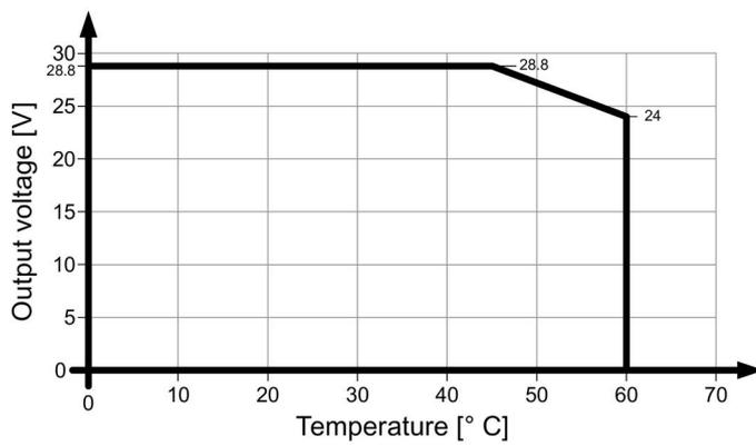
Figure 6-7 Output derating depending on the ambient temperature at  $I_{out rated}$
