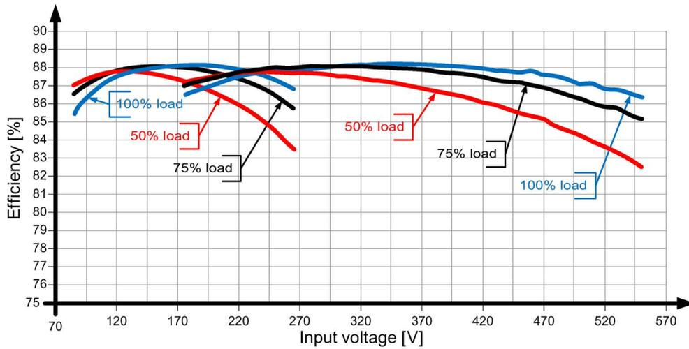
Figure 6-18 6EP1333-3BA10 efficiency
