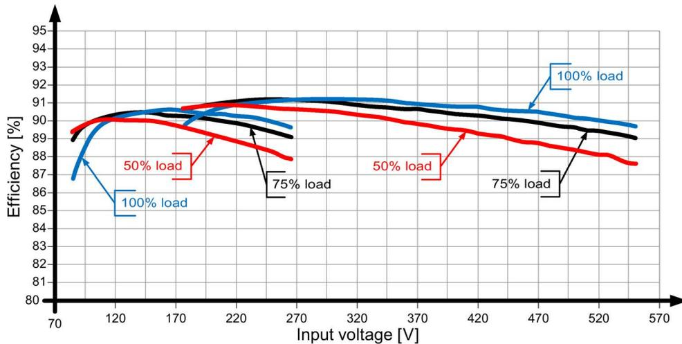
Figure 6-19 6EP1334-3BA10 efficiency
