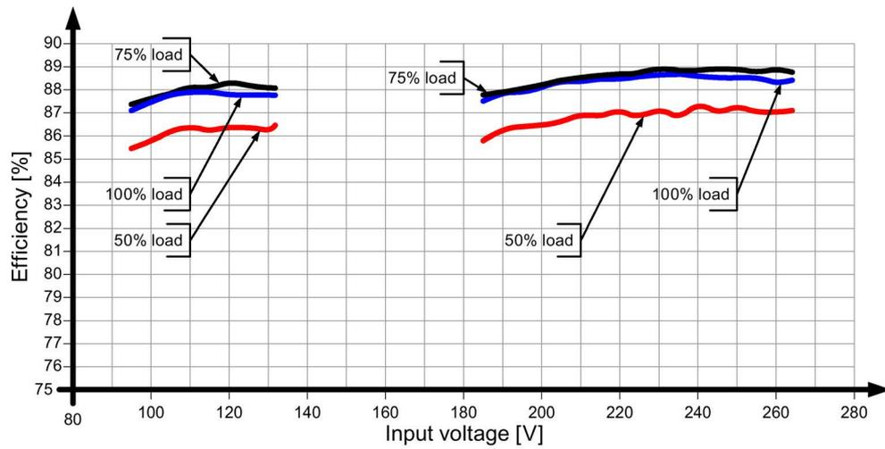
Figure 6-20 6EP1336-3BA00 efficiency
