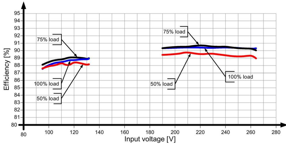
Figure 6-21 6EP1337-3BA00 efficiency
