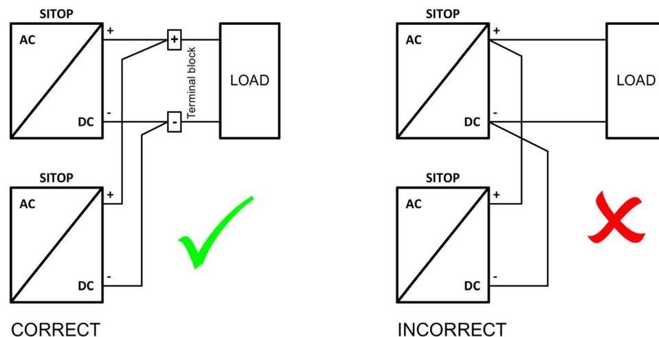
Figure 9-1 Parallel connection
