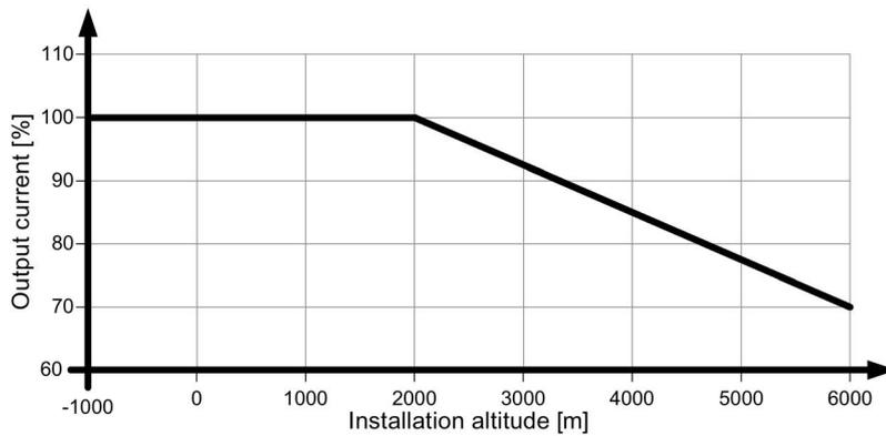
Figure 4-5 Mounting height derating
