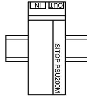
Figure 4-8 6EP1333-3BA10 mounting position (3)
