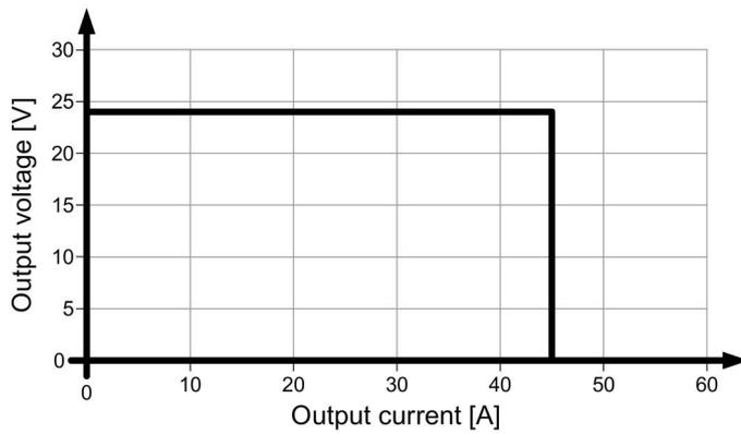
Figure 6-6 6EP1337-3BA00 single operation output characteristic
