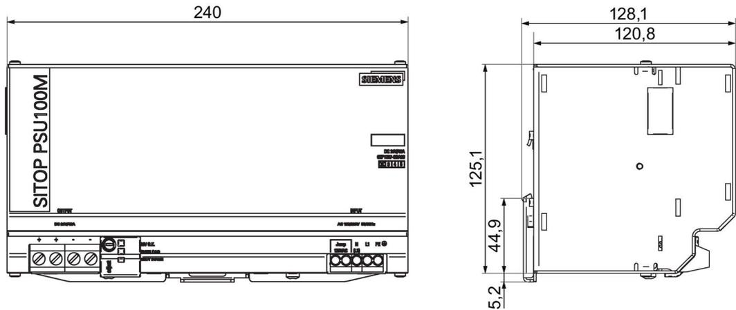
Figure 2-14 Dimension drawing for 6EP1337-3BA00
