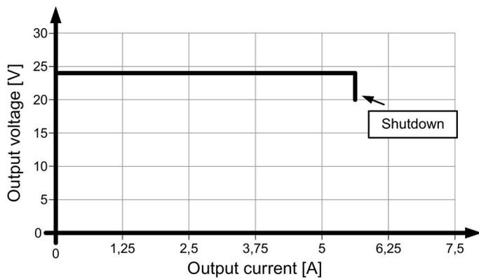
Figure 6-14 6EP1333-3BA10 latching shutdown output characteristic
