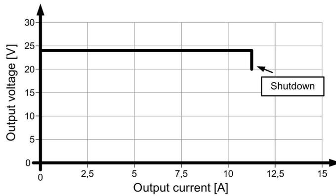
Figure 6-15 6EP1334-3BA10 latching shutdown output characteristic
