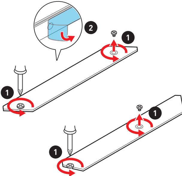
3. Move and fasten the M.2 standoff to the appropriate position for your M.2 SSD, or remove the M.2 standoff if your M.2 SSD length is same as the length of M.2 heatsink to avoid damage to the M.2 SSD.
