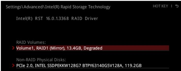
4. Select the **Degraded** RAID volume from the **Intel(R) Rapid Storage Technology** screen to enter the **RAID VOLUME INFO** screen.
